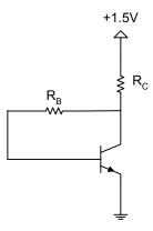
b) If  $\beta$  of the BJT happens to be 120, find the new Q point ( $I_C$ ,  $V_{CE}$ ). Use the values of  $R_B$  and  $R_C$  that you found in part (a).
